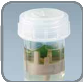
STEP 2 The mint leaves are combined with ethanol and are placed in a DT Tube.
